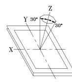
Inspection should be performed within  $\emptyset$  ( $\emptyset$ =30°) from Z axis to each X and Y axis.
